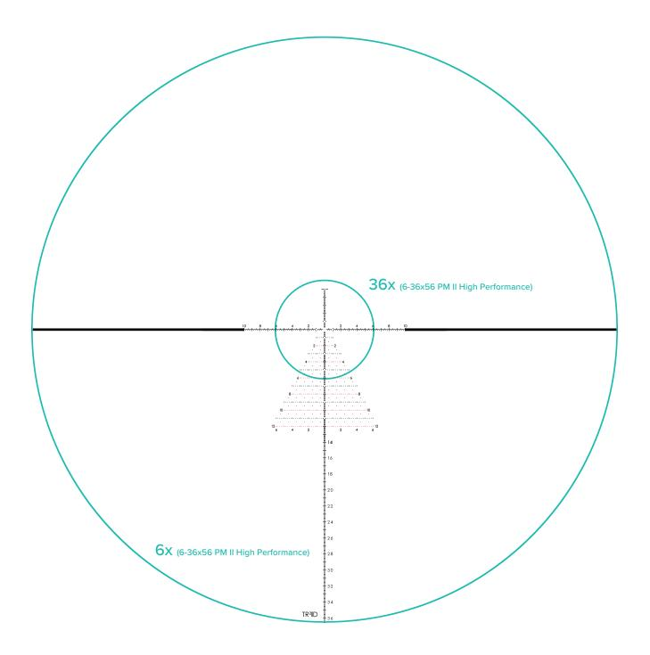
Field of View (FOV) The circles show the field of view of the particular magnifications
